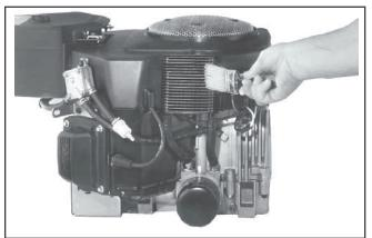
Figure 10. Blower Housing Mounted Oil Cooler.
