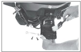
Figure 11. Cleaning Blower Housing Mounted Oil Cooler.
