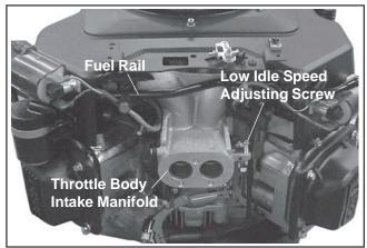
Figure 24. EFI Throttle Body Manifold.
