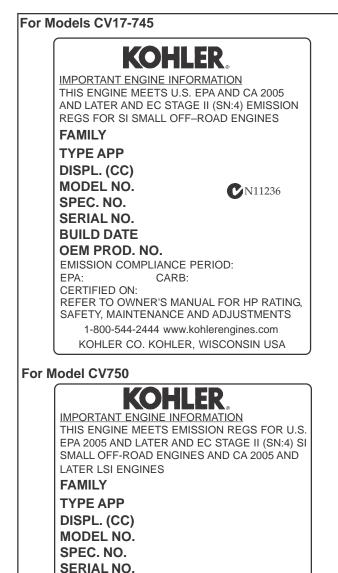
The Emission Compliance Period referred to on the Emission Control or Air Index label indicates the number of operating hours for which the engine has been shown to meet Federal and CARB emission requirements. The following table provides the Engine Compliance Period (in hours) associated with the category descriptor found on the certification label.
