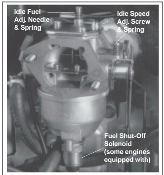
Figure 19. Carburetor CV17-25, CV675-740.
