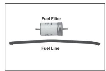
Figure 17. EFI Fuel Filter and Line.
