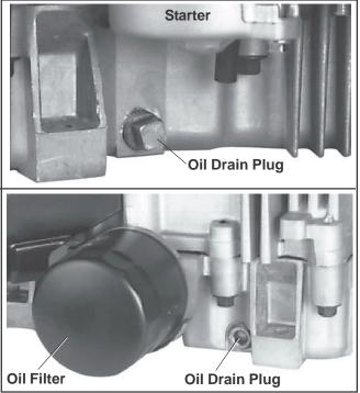
Figure 8. Oil Drain Plugs and Oil Filter.
