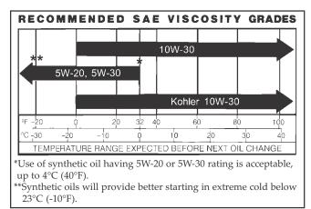
Figure 3. Viscosity Grades Table.
