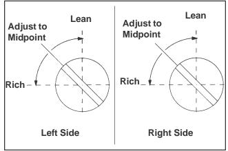
Figure 23. Optimum Low Idle Fuel Settings.
