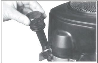
Figure 6. Checking Oil Level.
