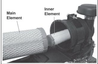
Figure 14. Removing Elements.
