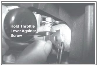
Figure 21. Holding Throttle Lever Against Idle Stop Screw.
