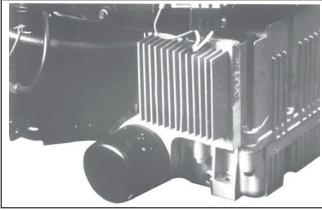
Figure 9. Crankcase Mounted Oil Cooler.
