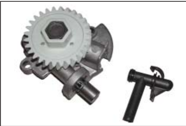
Figure 10-17. Oil Pump, Plastic Oil Pickup, and One-Piece Relief Valve (Later Style).
