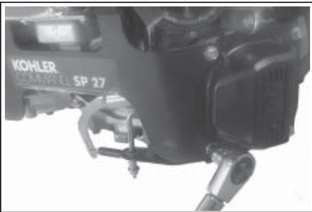
Figure 11-89. Securing Air Cleaner Mounting Bracket.
