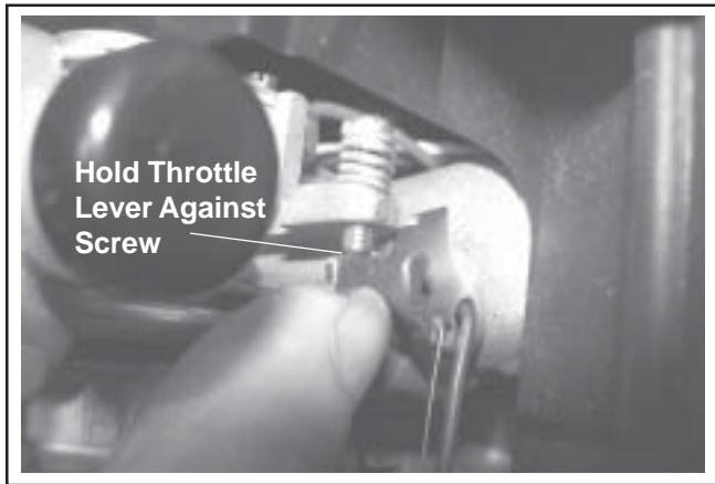
Figure 5-8. Holding Throttle Lever Against Idle Stop Screw (One-Barrel Carburetor).
