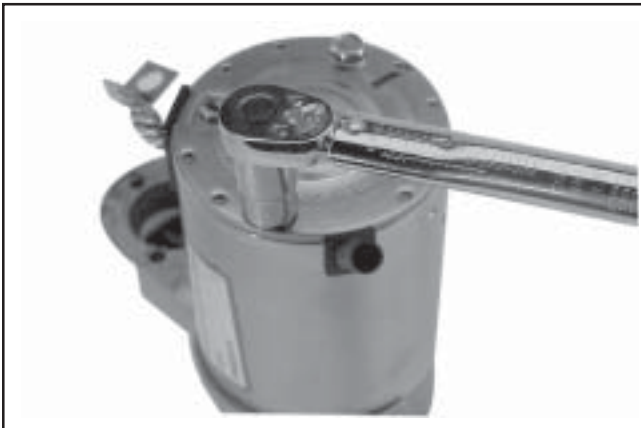
Figure 8-71. Torquing Thru Bolts.
