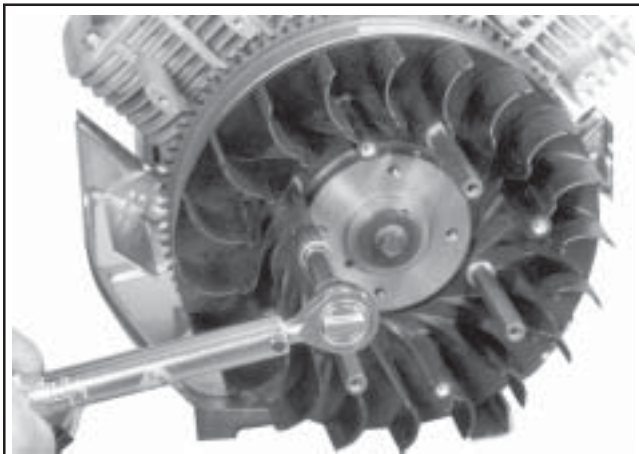
Figure 11-29. Torquing Supports for Metal Screen (Some Models).
