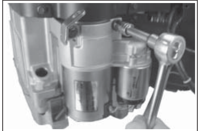
Figure 9-25. Removing Electric Starter Motor.
