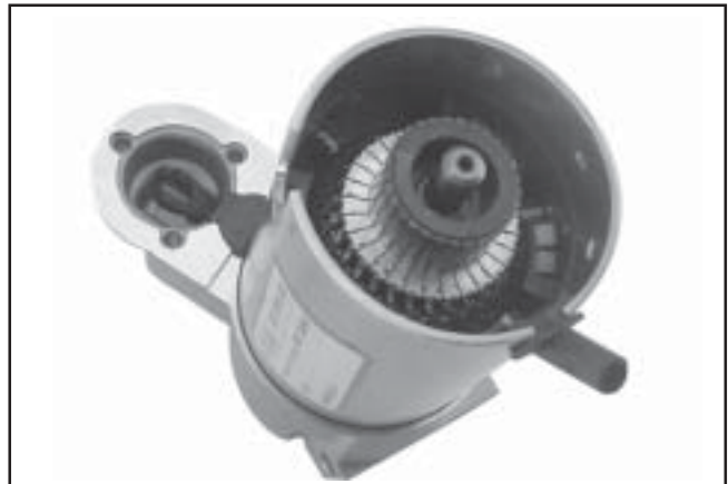
Figure 8-65. Installing Frame and Drain Tube.
