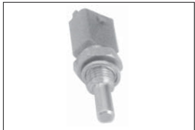
Figure 5B-8. Engine (Oil) Temperature Sensor.
