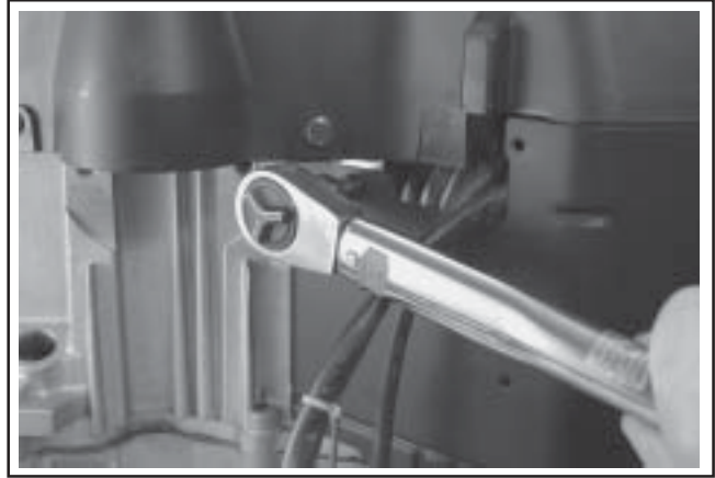
Figure 11-61. Tightening Short Screws for Outer Baffles.
