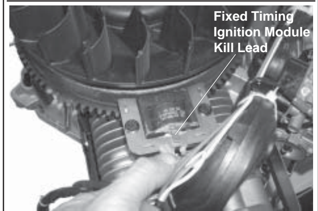
Figure 9-38. Disconnect Lead(s) from Ignition Modules.
