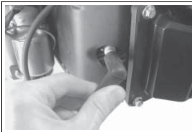
Figure 11-93. Connect Spark Plug Leads.
