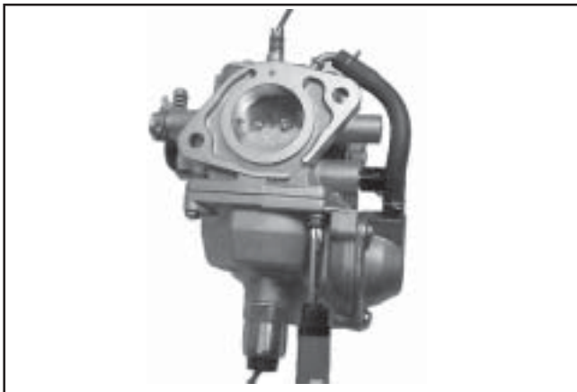
Figure 5-27. Installing Fuel Bowl.
