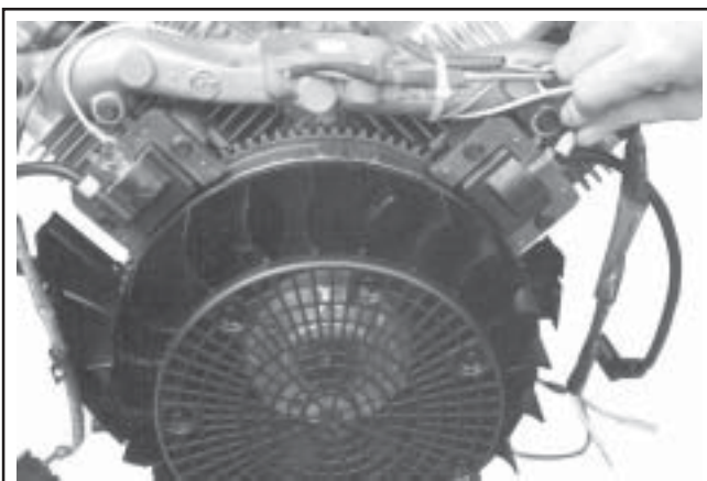
Figure 11-51. Connecting Kill Leads on Standard Ignition Modules.
