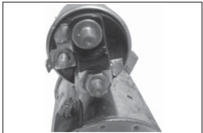
Figure 8-73. Positive (+) Brush Lead Connection.
