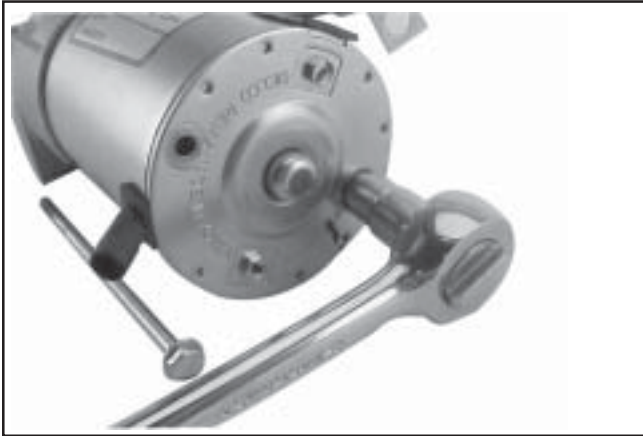
Figure 8-48. Removing Thru Bolts.
