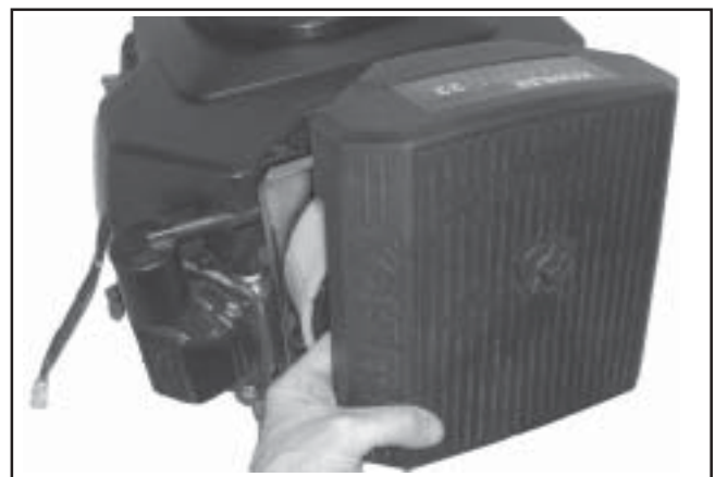
Figure 9-5. Removing Standard Air Cleaner Cover.
