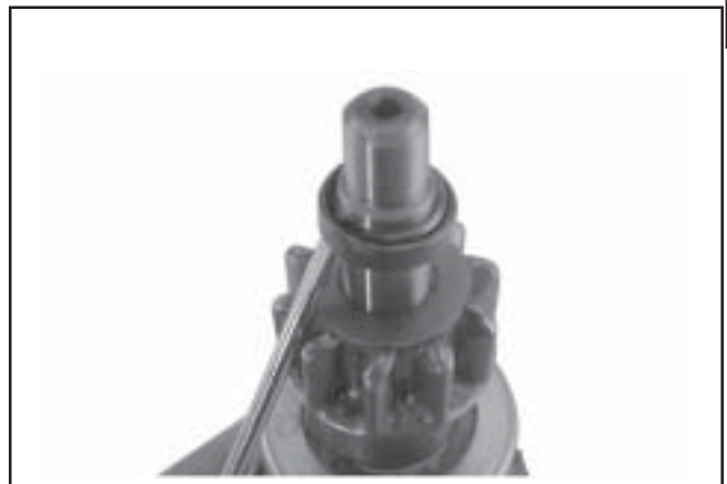
Figure 8-61. Installing Stop Collar and Retainer.
