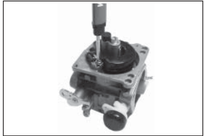
Figure 5-24. Installing Float Assembly.
