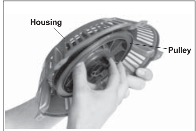
Figure 7-6. Removing Pulley from Housing.
