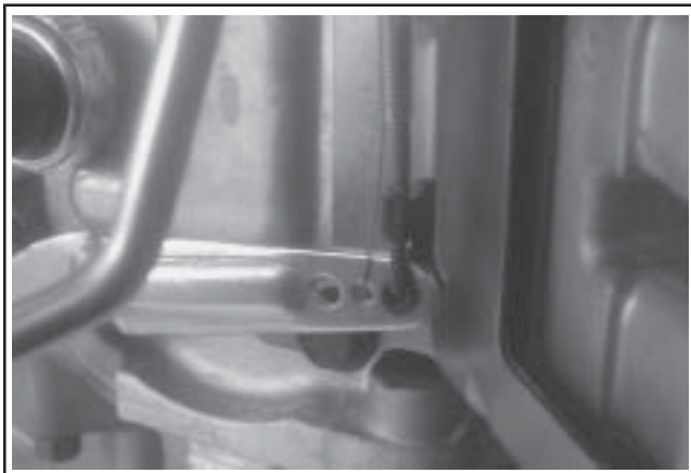
Figure 11-73. Throttle Linkage Details.
