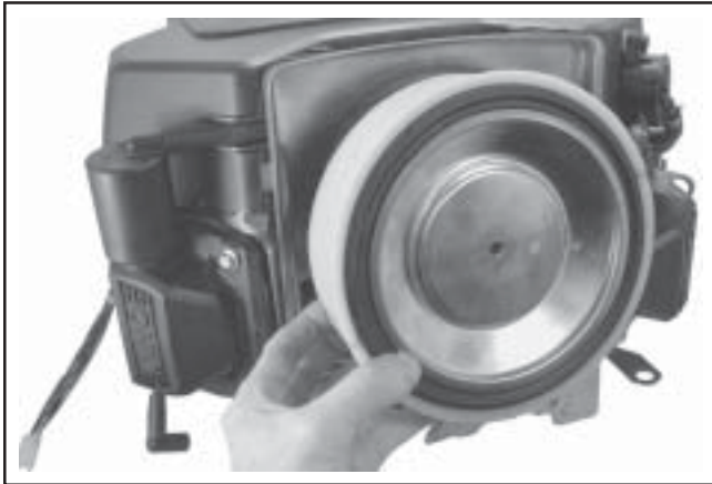
Figure 9-6. Removing Standard Element and Precleaner.
