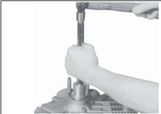
Figure 11-2. Installing Oil Seal in Crankcase.
