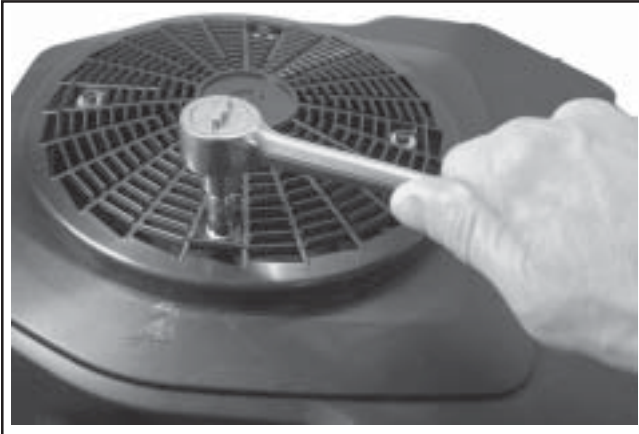
Figure 9-30. Removing Flywheel Screen.
