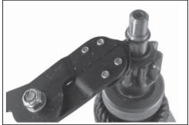
Figure 8-54. Removing Retaining Ring.
