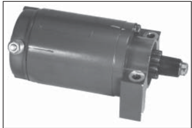
Figure 8-41. Starter Assembly Match Marks.
