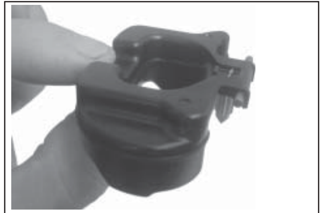
Figure 5-45. Float and Inlet Needle Details.
