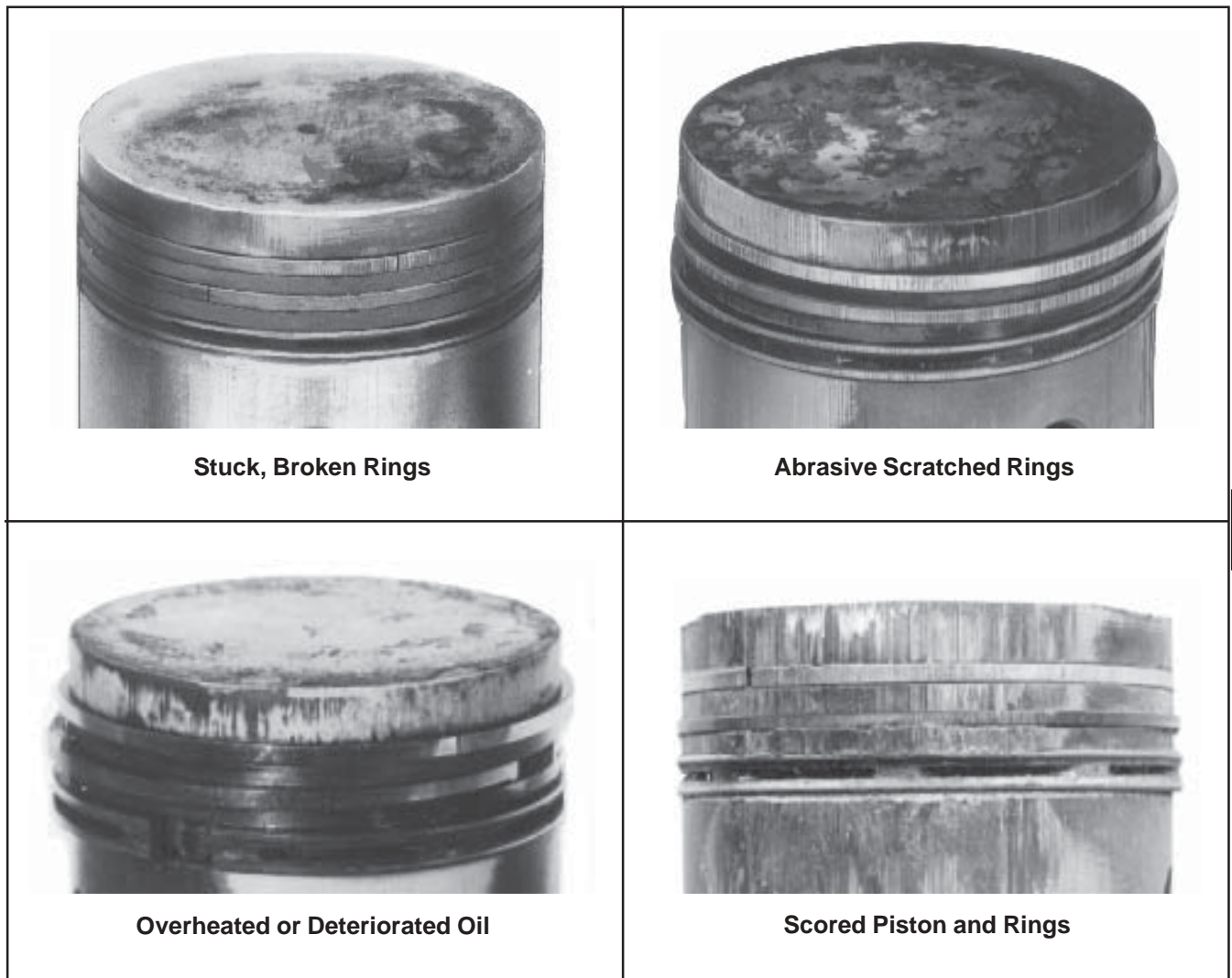
Figure 10-8. Common Types of Piston Damage.
