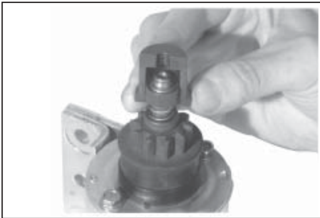
Figure 8-38. Assembling Larger Inner Half Around Spring Retainer.
