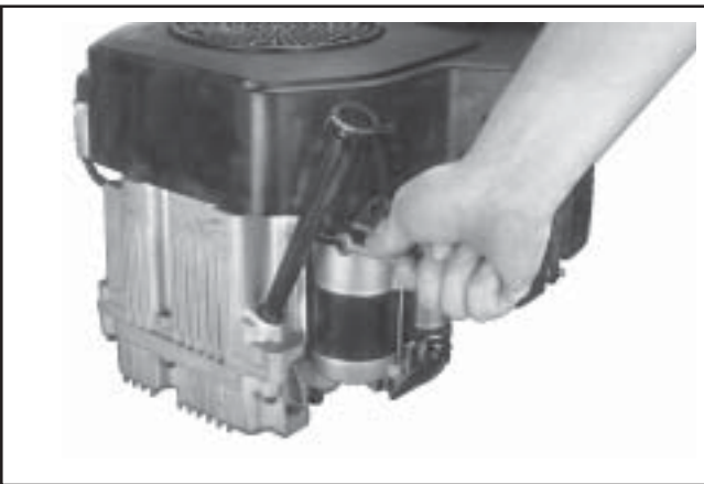
Figure 9-3. Removing Oil Fill Tube Bracket.
