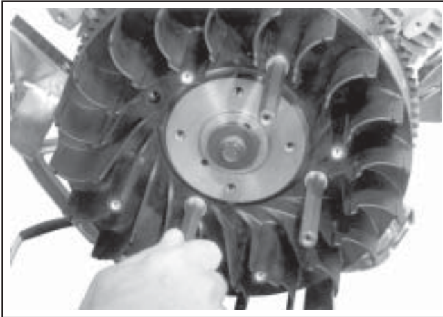
Figure 11-28. Installing Supports for Metal Grass Screen.
