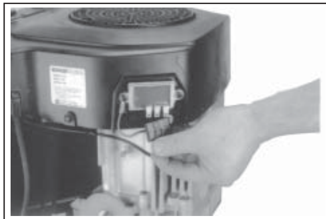
Figure 11-65. Attaching Connector Plug.
