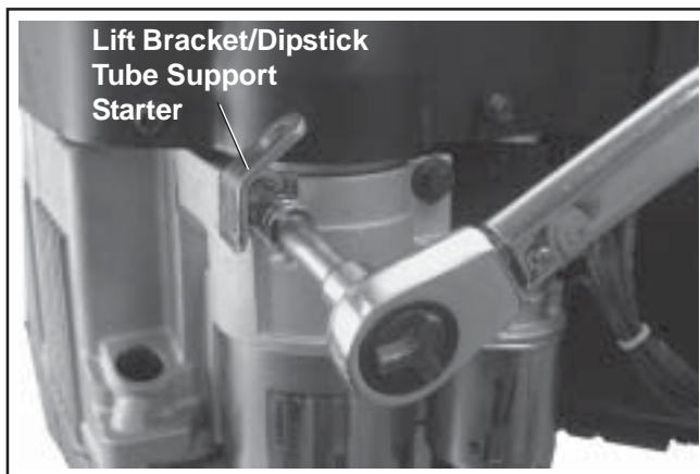
Figure 11-79. Installing Starter and Lift Bracket.
