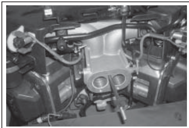
Figure 5B-32. Upper Throttle Body/Intake Manifold Details.
