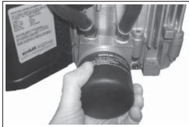
Figure 11-91. Installing and Tightening Oil Filter.
