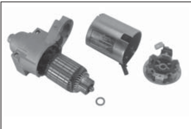
Figure 8-50. Starter Frame Removed.
