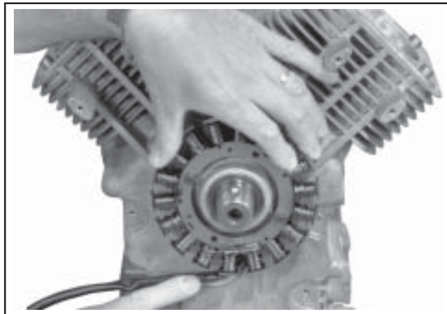
Figure 11-21. Route Stator Leads in Groove.
