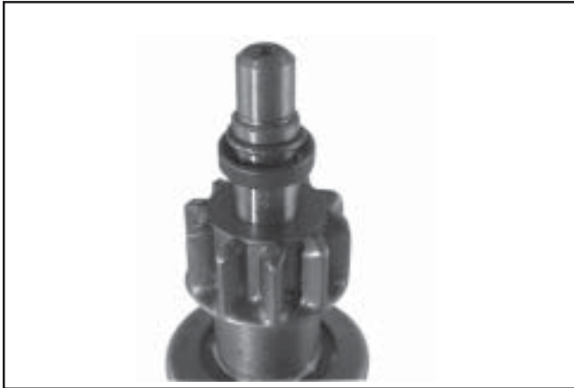
Figure 8-53. Retaining Ring Detail.
