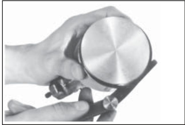
Figure 10-10. Measuring Piston Ring Side Clearance.
