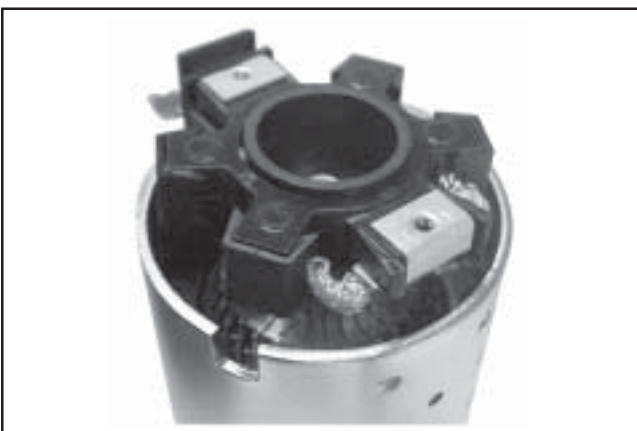
Figure 8-67. Installing Brush Holder Assembly with Supplied Tube.
