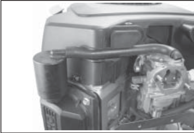
Figure 11-84. Breather Hose and Separator Details.
