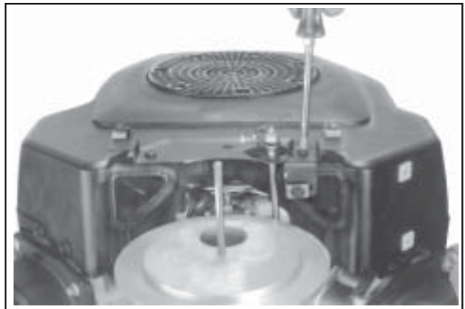
Figure 11-75. Installing Control Panel.
