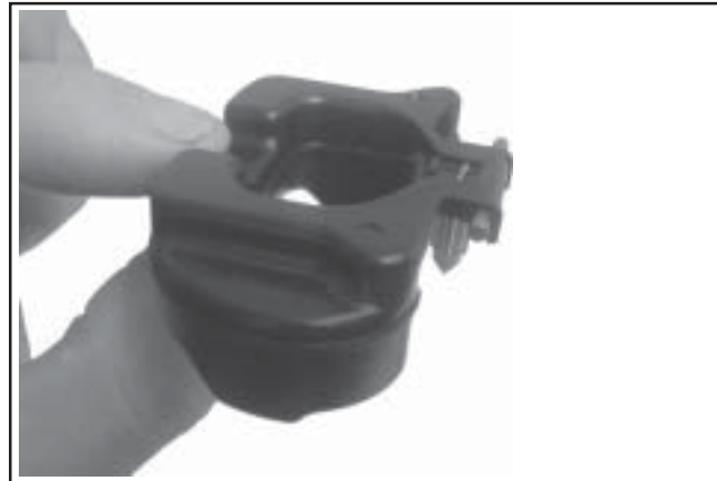
Figure 5-56. Float and Inlet Needle Details.
