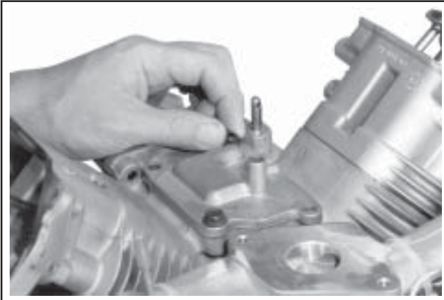
Figure 11-54. Installing Screws (Locations 3 and 4).
