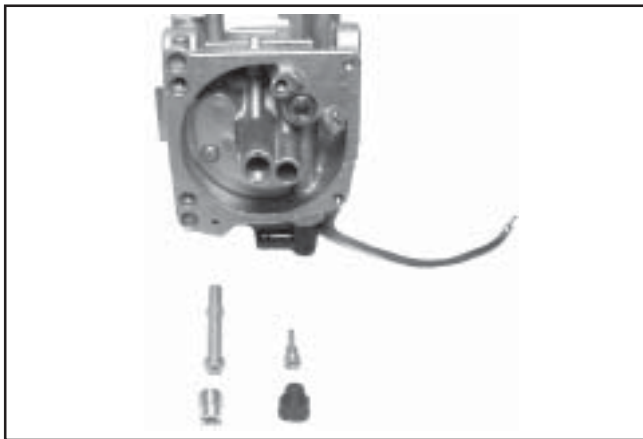
Figure 5-19. Main Jet and Slow Jet Removed.
