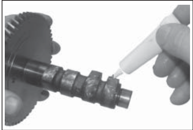
Figure 11-12. Apply Camshaft Lubricant to Cam Lobes.
