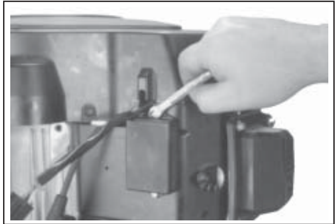
Figure 9-27. Loosening Spark Advance Module (Applicable Models).
