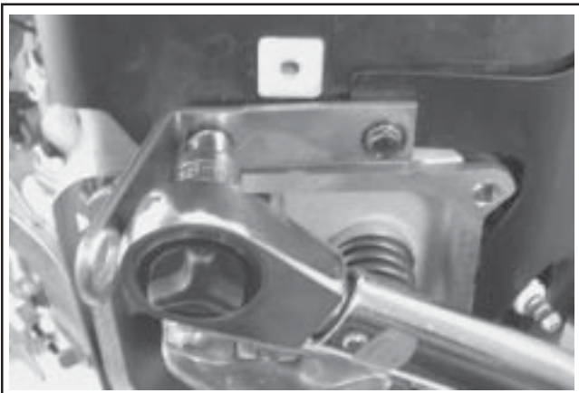
Figure 11-60. Tightening Outer Baffle Front Screws.
